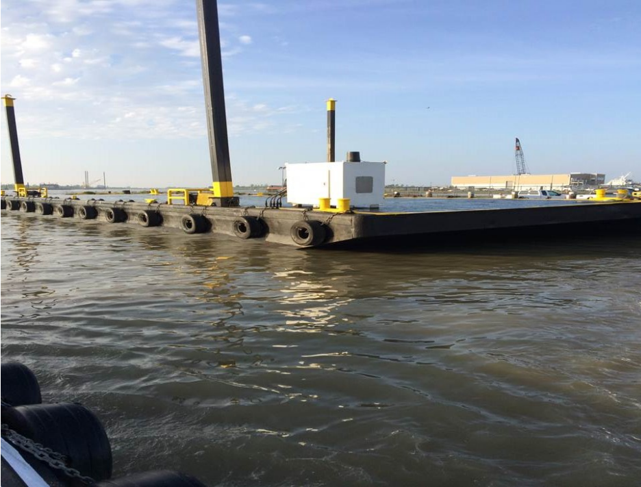
Diesel pulling unit (2) 35'x16" Square Spuds
