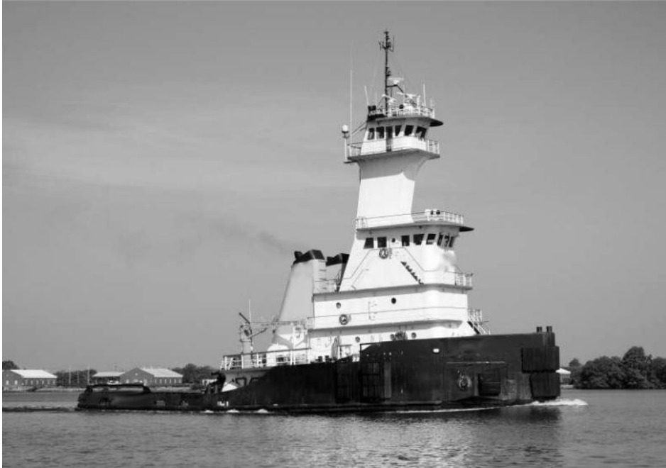
Elevated pilothouse with elevator access, fitted with rudder fendering designed for towing in the notch.
