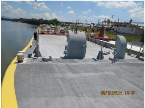
• Tanks per Barge: 6 Tank Thickness:1 1/4" • Tank Length: 68' 4 'A"
